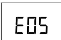
The unit will be displaying "EO5" if the self-test fails three consecutive times.
