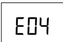
If the unit is displaying "EO4", the battery voltage will be too low or below a certain level when 3 hours passed.
