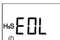
If the unit is displaying "**EOL**", the life remaining of the unit will be less than 8 hours.
